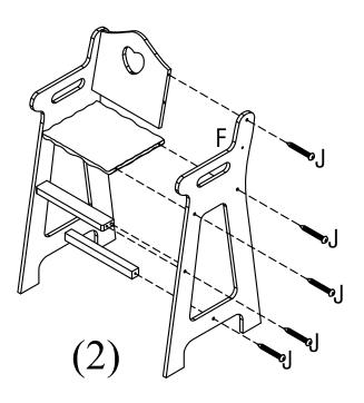
The countersunk holes on the side panels face out when assembled. So, this determines which panel is left and which is right.
