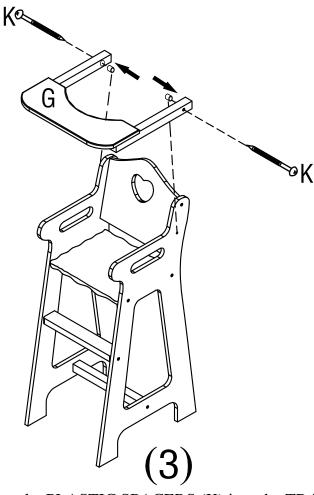
In STEP 3, insert the PLASTIC SPACERS (K) into the TRAY ARMS (G) first, and then attach the TRAY (G) to the SIDES (B and F) using the LONG SCREWS (K).
