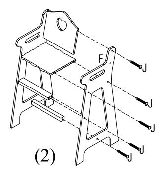
The countersunk holes on the side panels face out when assembled. So, this determines which panel is left and which is right.
