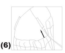
6. Thread the (H x 2) Canopy Rods through the fabric guide channels on the (I x 1) Fabric Canopy with Drapes. They will cross in the center like a 'X'.
