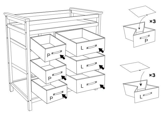
LARGE AND SMALL BASKETS CAN BE INSERTED FROM EITHER SIDE OF THE TABLE SO THAT YOU CAN CHOOSE TO HAVE THE LARGE BASKETS ON THE LEFT AND SMALL BASKETS ON THE RIGHT OR VICE VERSA, DEPENDING ON WHICH SIDE OF THE TABLE FACES FRONT. THE BASKETS ARE ALSO REVERSIBLE COLOR SO YOU CAN CUSTOMIZE THE LOOK OF YOUR TABLE.
