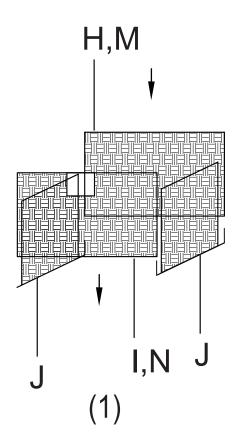
NOTE: The prongs on PARTS J must be fitted into the openings on PARTS H, I, M and N.
